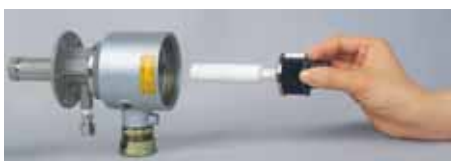
Easily replaceable zirconia element
